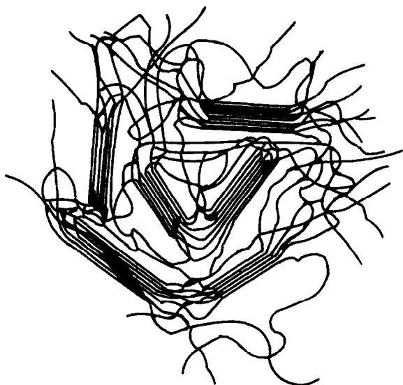
Fig. 8. Diagrammatic representation of the fringed micelle model of polymer crystallinity (Van Krevelen, 1976).
